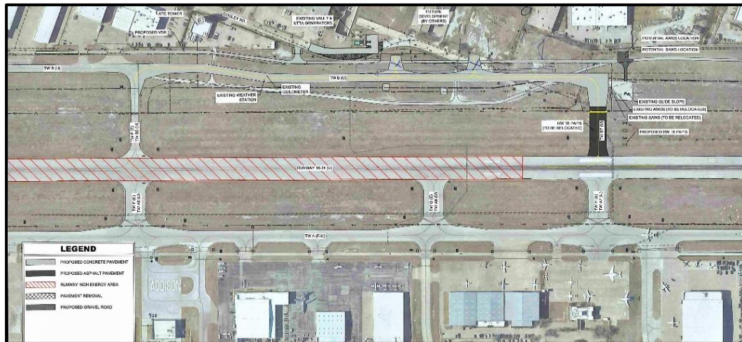
Left: extensions of Taxiway Bravo and Taxiway Hotel
