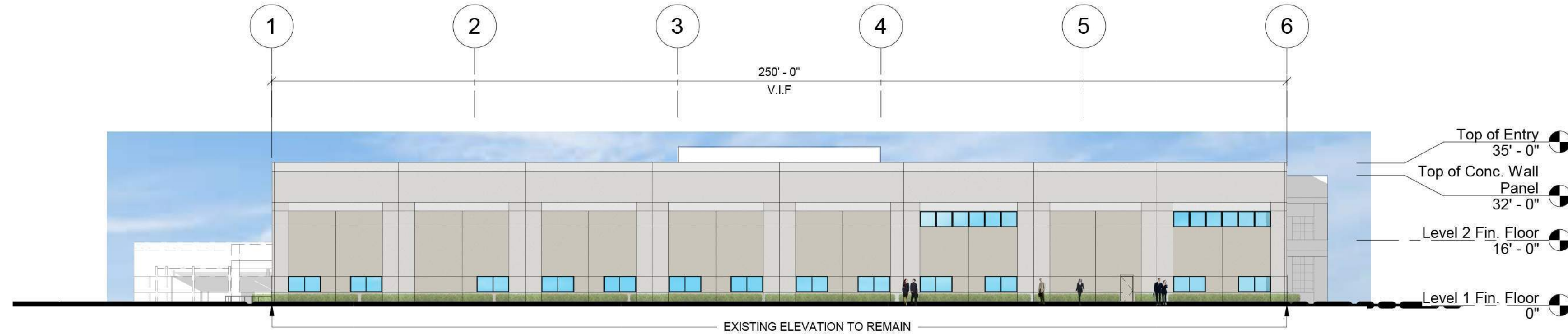
03 EXISTING ELEVATION SOUTH SCALE: 3/64" = 1'-0"
