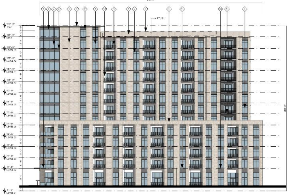
1 MULTI-FAMILY HR - OPT 1 - WEST ELEVATION SCALE: 1/16" = 1'-0"
