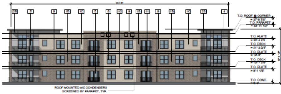
04 BLDG #2 - NORTH ELEVATION (FRONT) SCALE: 1/8" = 1'-0"
