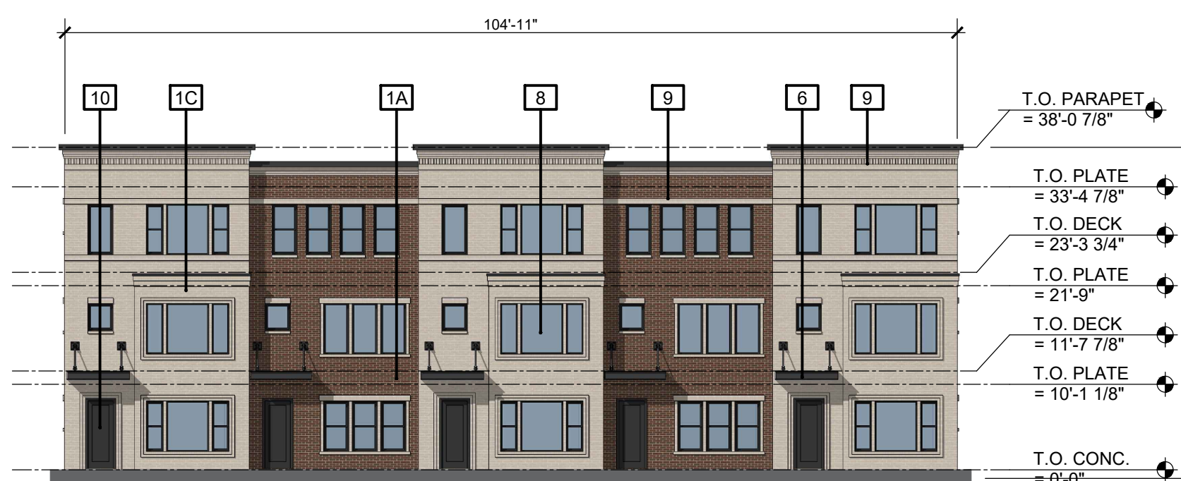
01 BLDG #3&4 - WEST ELEVATION SCALE: 1/16" = 1'-0"
