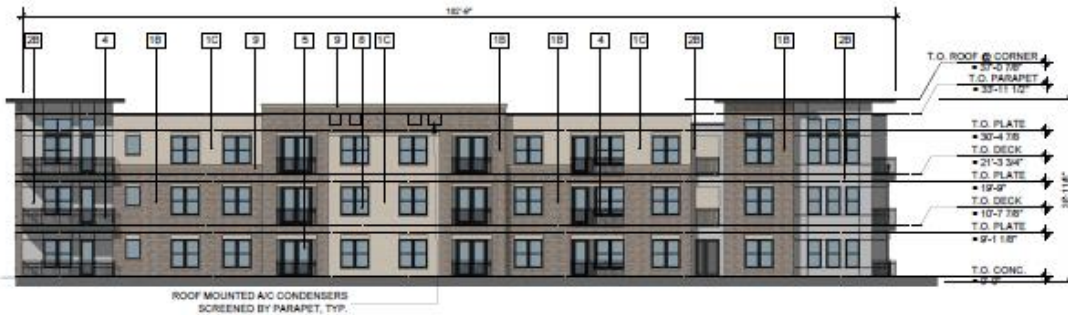
02 BLDG #2 - EAST ELEVATION SCALE: 1/8" = 1'-0"
