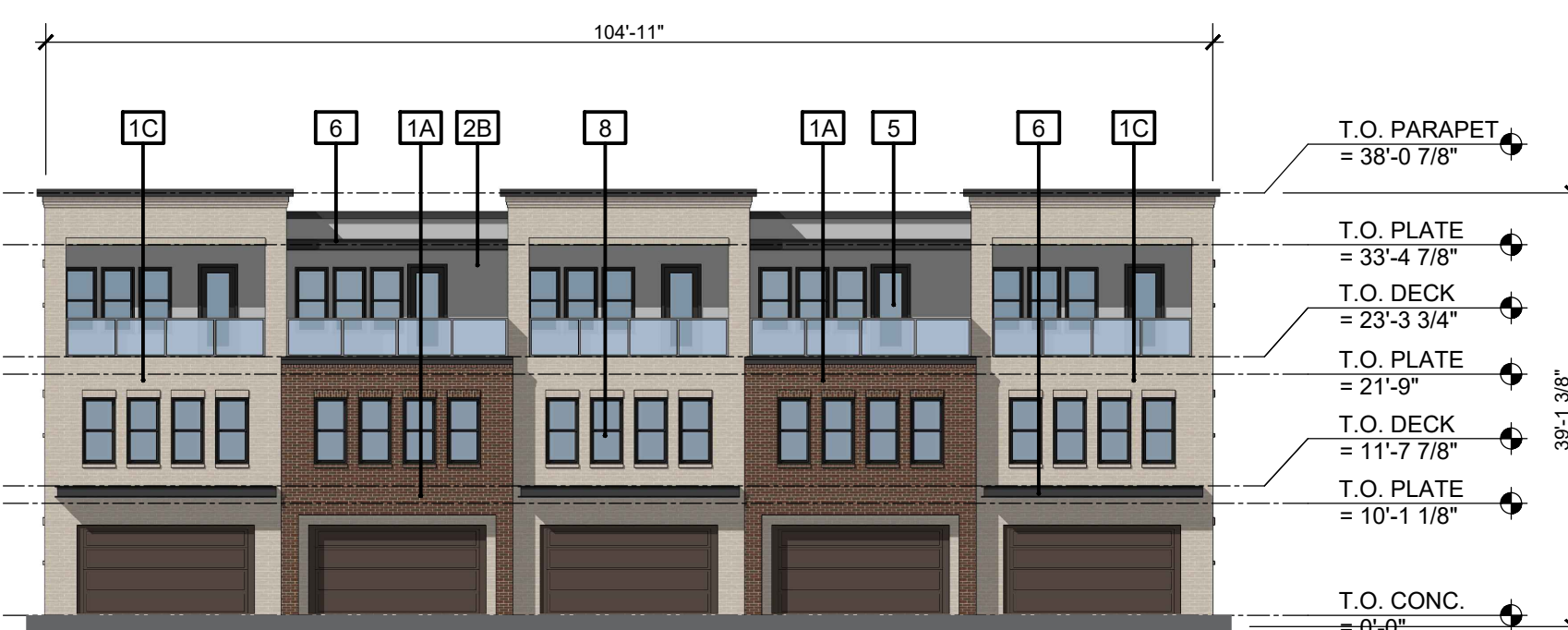
02 BLDG #3&4 - EAST ELEVATION SCALE: 1/16" = 1'-0"
