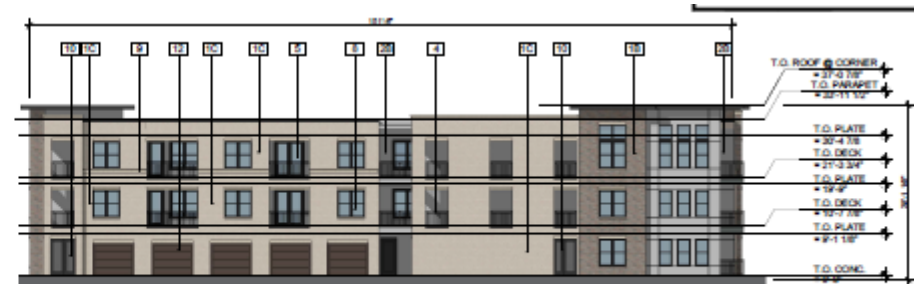
03 BLDG #2 - SOUTH ELEVATION SCALE: 1/8" = 1'-0"
