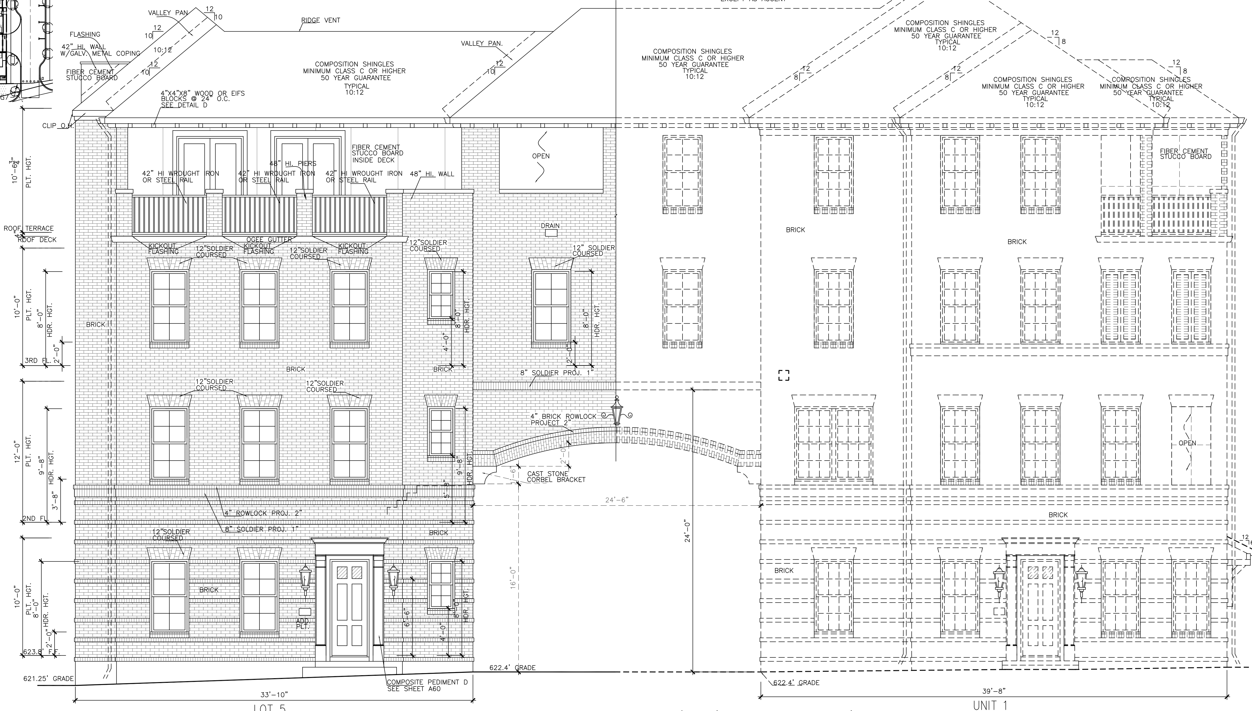
LOT 5 BUILDING 12 west/front(HOLLY STREET) elevation SCALE: 1/4" = 1'-0"
