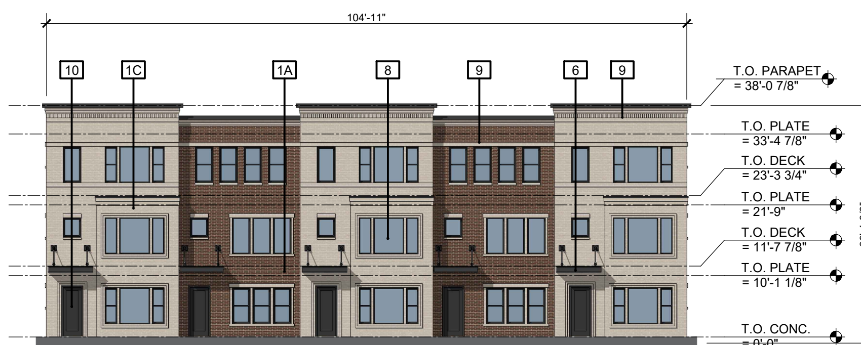
01 BLDG #3&4 - WEST ELEVATION SCALE: 1/16" = 1'-0"
