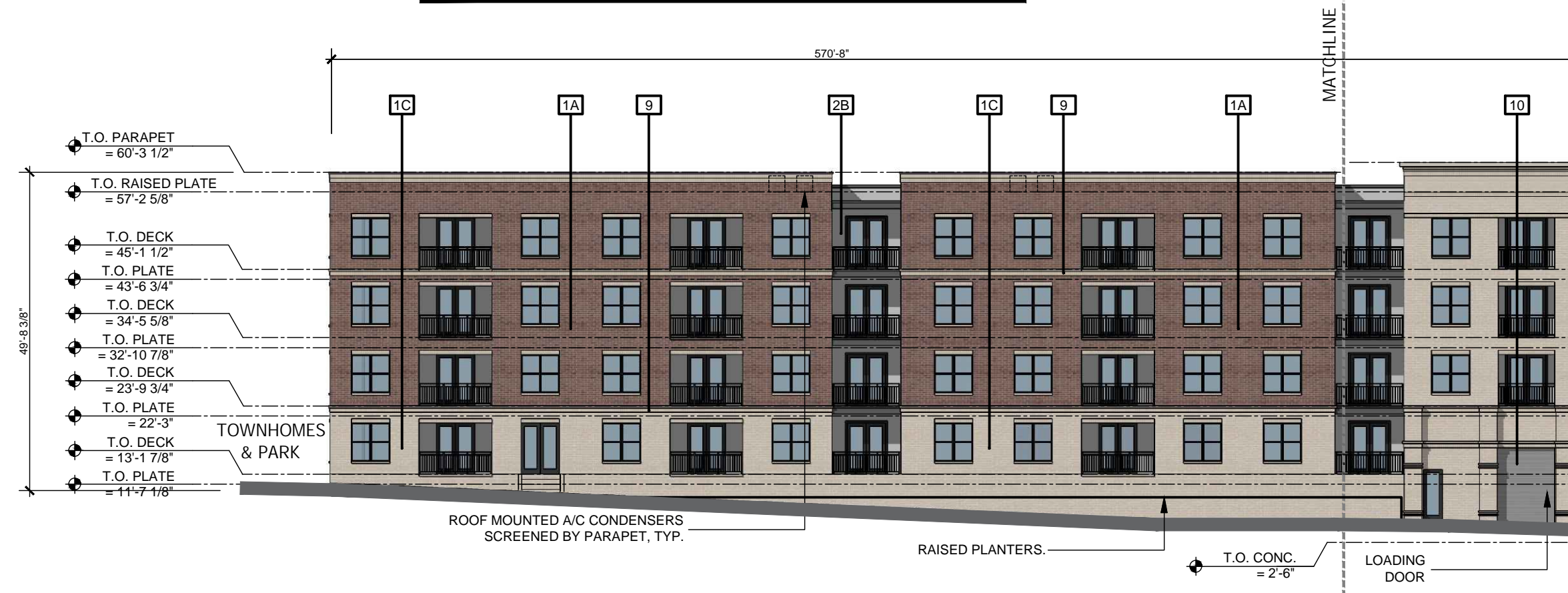
03 BLDG #1 - SOUTH ELEVATION SCALE: 1/8" = 1'-0"
