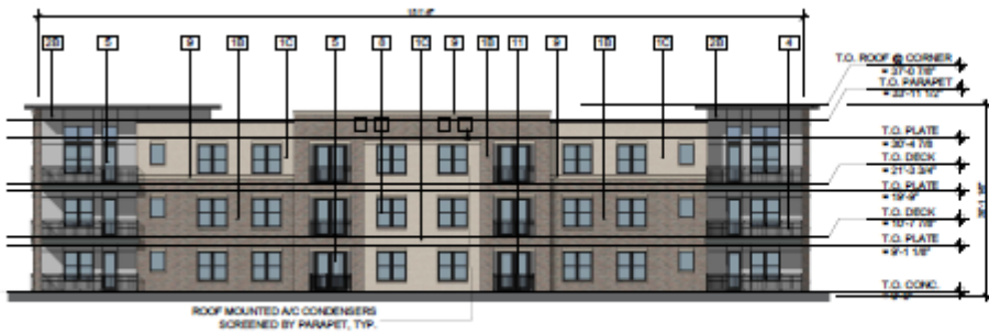
04 BLDG #2 - NORTH ELEVATION (FRONT) SCALE: 1/8" = 1'-0"
