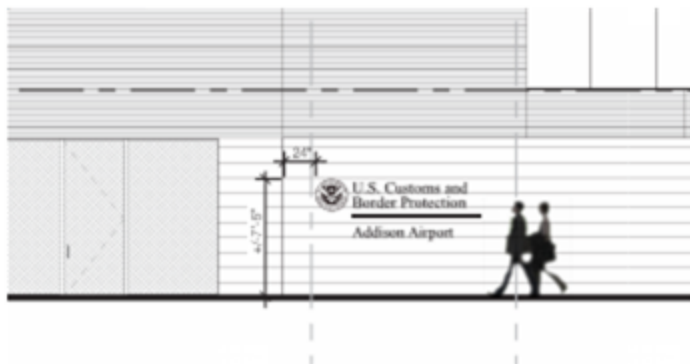
Location 004 South Elevation, Ground Level Location to be verified in field for alignment to wall panel seaming and spacing from wall end prior to installation.
