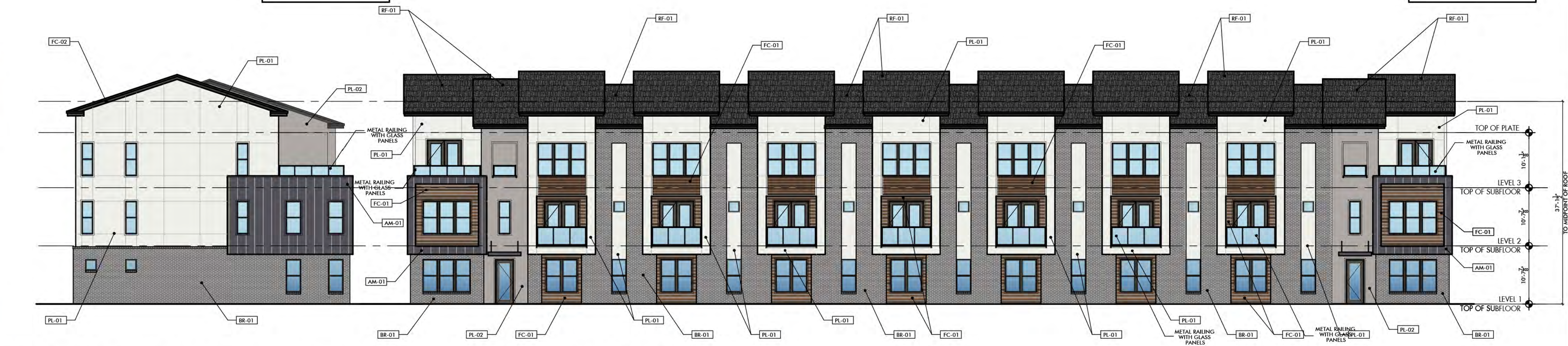
NORTH ELEVATION (MAIN ENTRY) SCALE: 3/32" = 1'-0"
