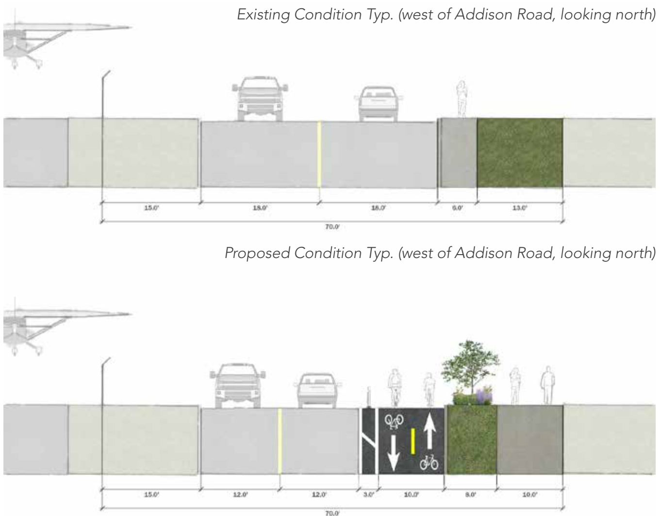
Figure 5-9: Westgrove Drive Cycle Track and Wide Sidewalk
