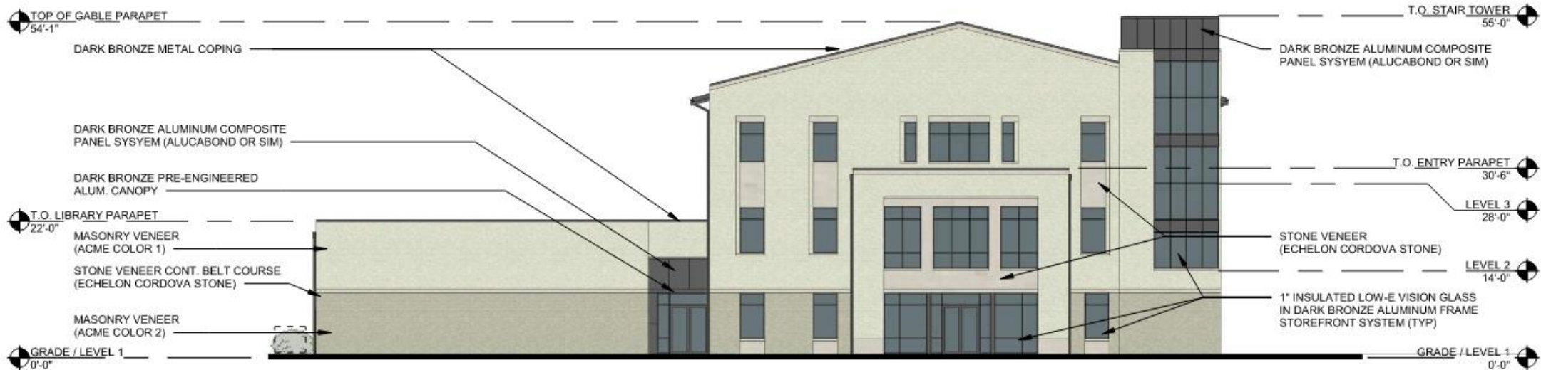
04 SOUTH ELEVATION (FRONT) 1/16" = 1'-0"
