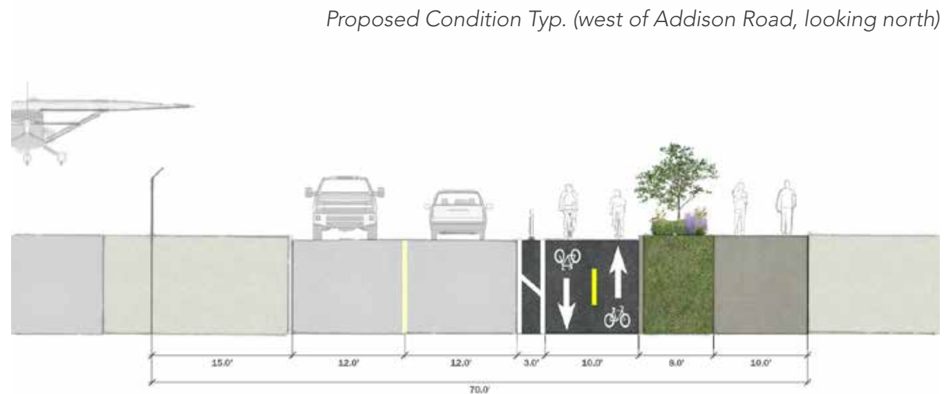
Figure 5-9: Westgrove Drive Cycle Track and Wide Sidewalk
