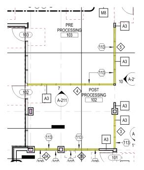
These walls have glass and aluminum framing that takes up the top half of the wall which does not allow the stud framing to run continuously from floor to deck above which compromises is integrity. See interior elevation shown below from sheet A-211 for quick reference:
