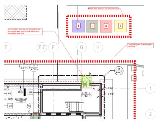
The originally specified hardware set for this door contained a panic device on the interior side per code requirements but was noted to not have any exterior lever/handle, cylinder, or
