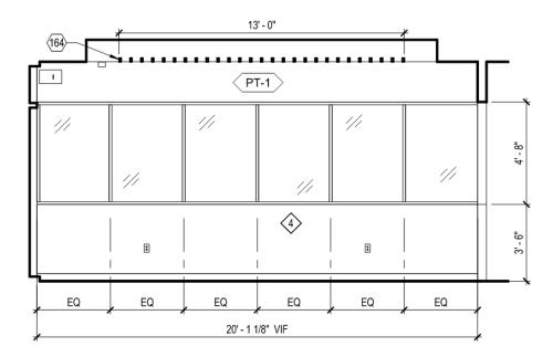
The wall support elements were installed below the windows inside the 3'-6" tall section of drywall framing to brace the wall from overturning/folding if a lateral force is applied to it in the middle of the wall.
