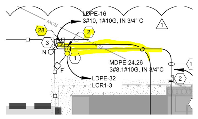
From electrical drawing - ES -102. items to be removed from the scope of work as mentioned in the list above.
