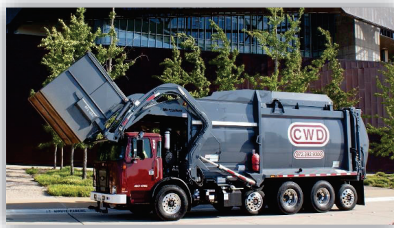
CWD front load truck servicing an eight-yard can
