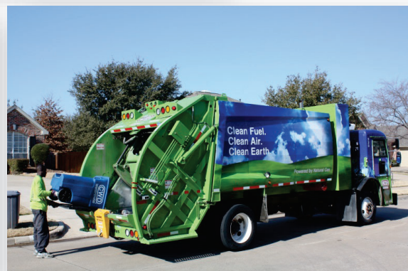
CNG Rear Load servicing recycling in Corinth
