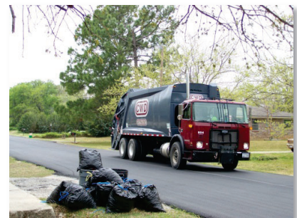
Rear load vehicle facilitates hand load collection
