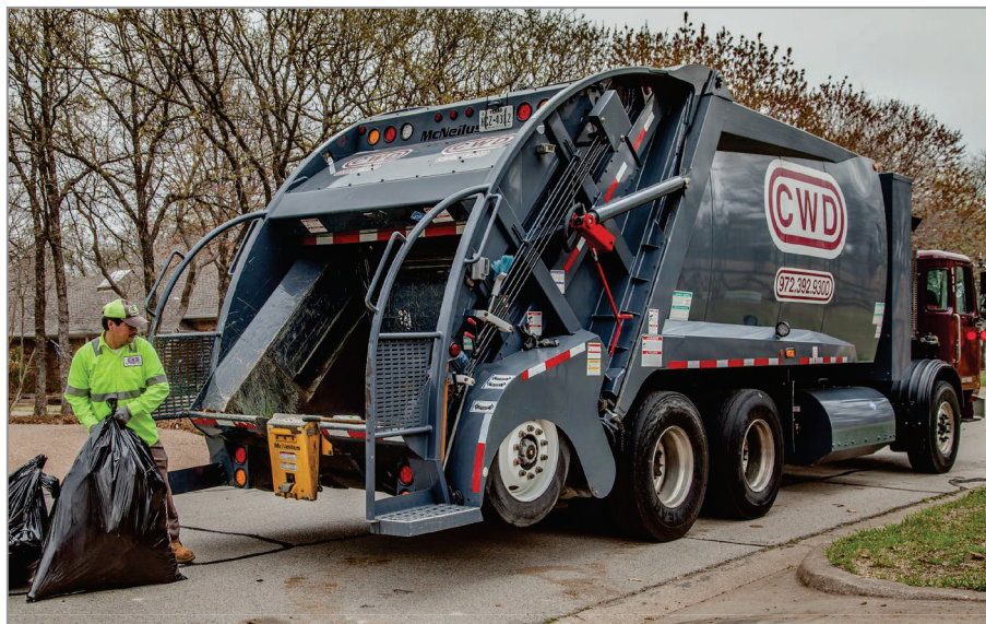
CNG Semi-Automated Rear Load Vehicle used for trash/recycle collection
