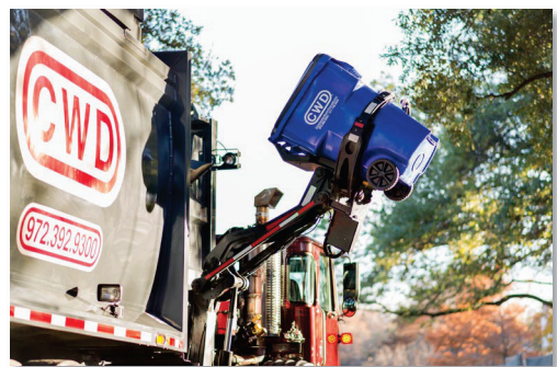
Automated Side Load (ASL) service
