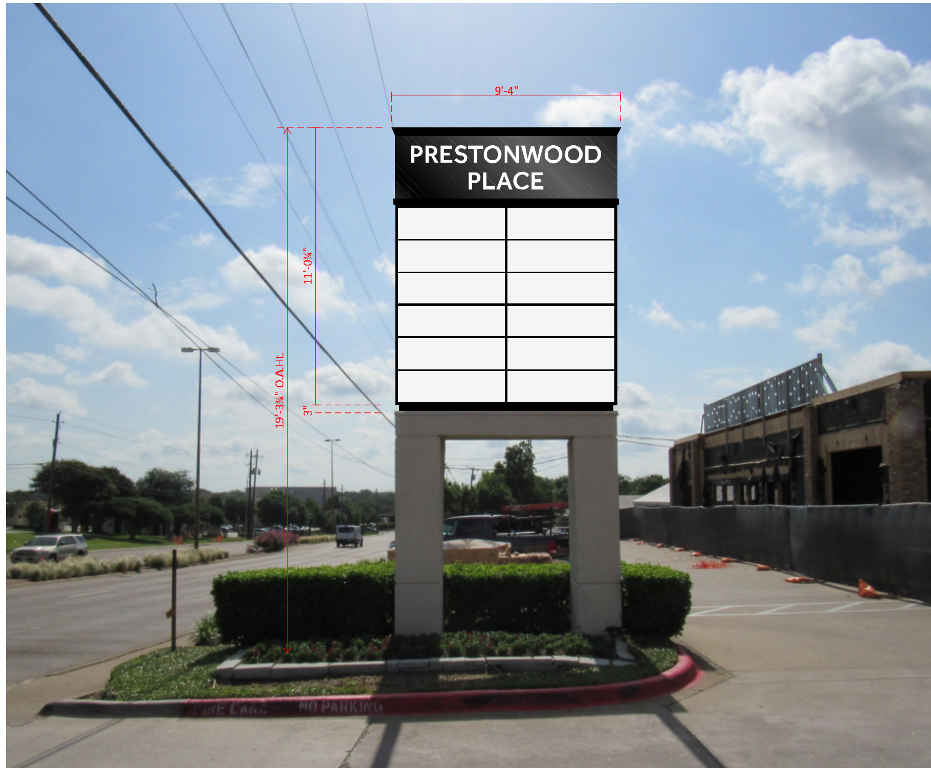
A1 PROPOSED NEW D/F PYLON SIGN CABINET
