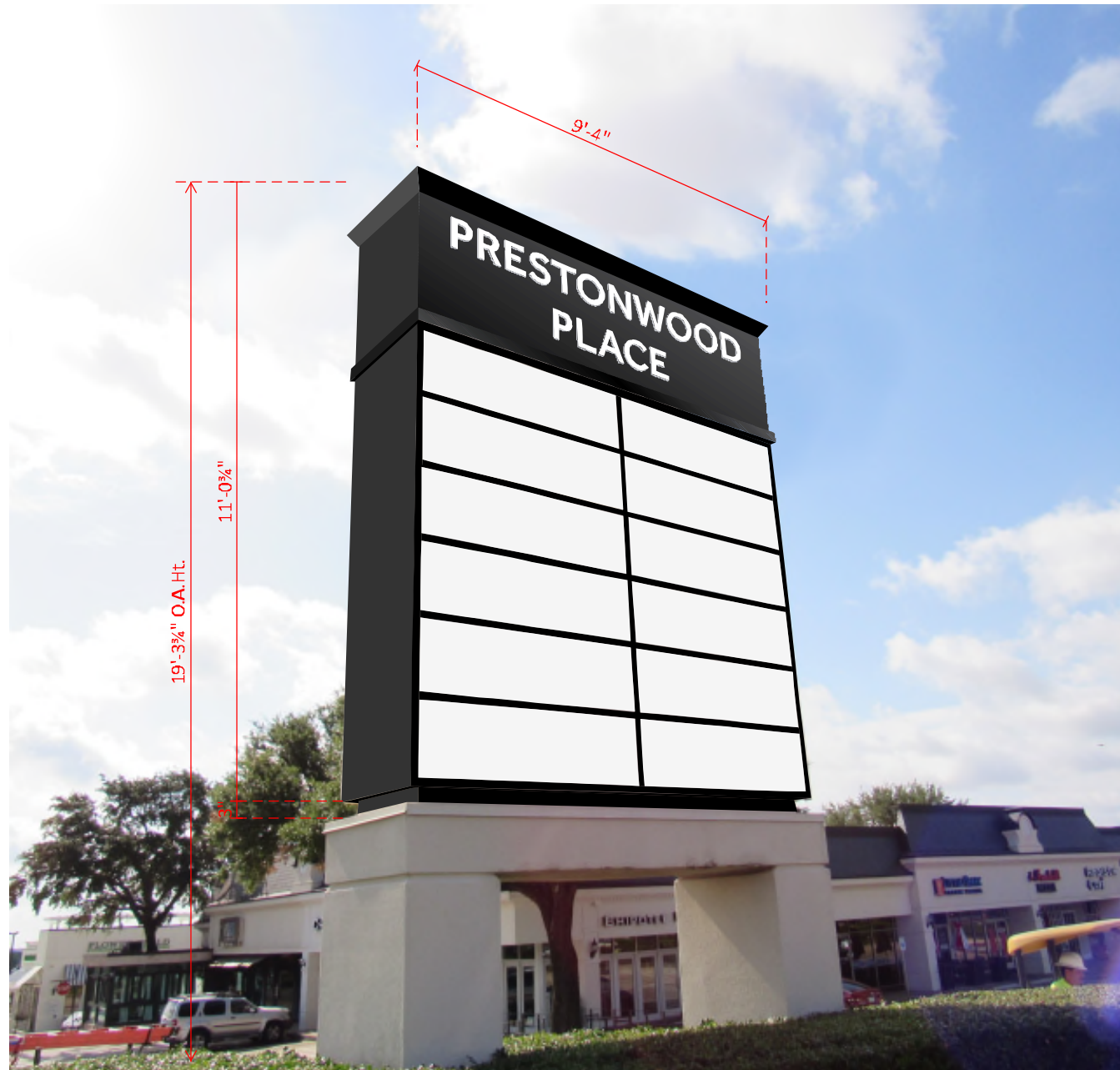
A2 PROPOSED NEW D/F PYLON SIGN CABINET
