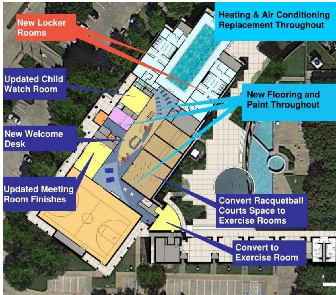
PROPOSED FIRST FLOOR PLAN
