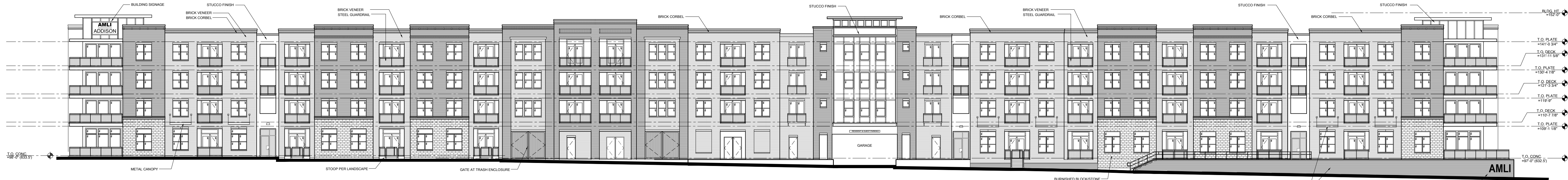
01 SPECTRUM DR. (EAST) ELEVATION SCALE: 1" = 20'-0" 90% BRICK/STONE VENEER 10% STUCCO FINISH MATERIAL
