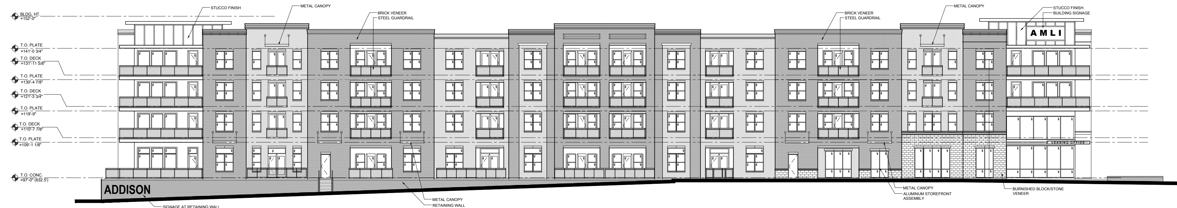
02 EDWIN LEWIS DR. (NORTH) ELEVATION SCALE: 1" = 20'-0" 95% BRICK/STONE MATERIAL 5% STUCCO FINISH MATERIAL
