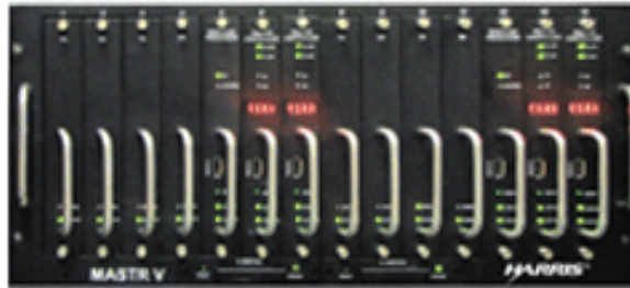
Figure 5. MASTR V Repeater Shelf with 4 RF Channels
